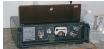
Figure 7 View of electrochemical analyser Istran EcaFlow GP 130
