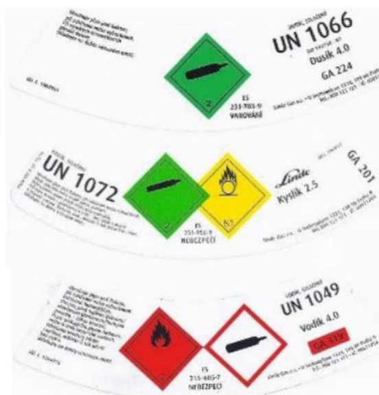
Figure No. 4: Types of precautionary labels for inert, combustion supporting and flammable gases
