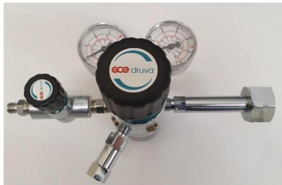
Figure No. 13: Double-stage pressure regulator
