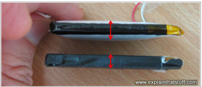
Photo: Lithium-ion (Li-ion) batteries can inflate like little cushions if they don't have a means of venting any gases produced during charging (mainly carbon monoxide, carbon dioxide, and hydrogen, though smaller amounts of other organic gases may also be present). Here are two identical batteries from a cellphone, the top one of which has almost doubled in width due to the trapped gases inside.
