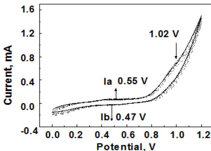
**Figure 4.** Cyclic voltammogram of a  $1 \times 10^{-3}$  mol L<sup>-1</sup> solution of **6** in CH<sub>3</sub>CN/ 0.2 mol L<sup>-1</sup> tetrabutylammonium fluoroborate +  $1 \times 10^{-3}$  mol L<sup>-1</sup> HCl on a Pt electrode. The electrode potential was swept repeatedly between 0 and 1.2 V vs. Ag/AgCl at a scan rate of 50 mV s<sup>-1</sup>.
