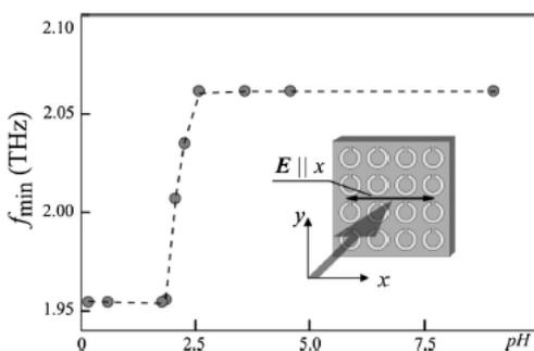
Fig. 4 pH-dependence of the red-shift of the transmission minimum
