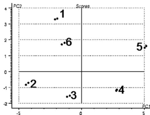
**Fig. 4** PCA score plot showing the ability of the electrode array to distinguish the Czech beers of different brands. The recognition pattern was measured with the following beer samples: 1 Bernard 10°, 2 dark Kozel 10°, 3 Kozel 10°, 4 Bráník 10°, 5 Radegast, 6 Staropramen ( $n = 5$ ). These measurements were carried out in thermostated cell at 25°C. The tested electrodes were washed with distilled water between measurements
