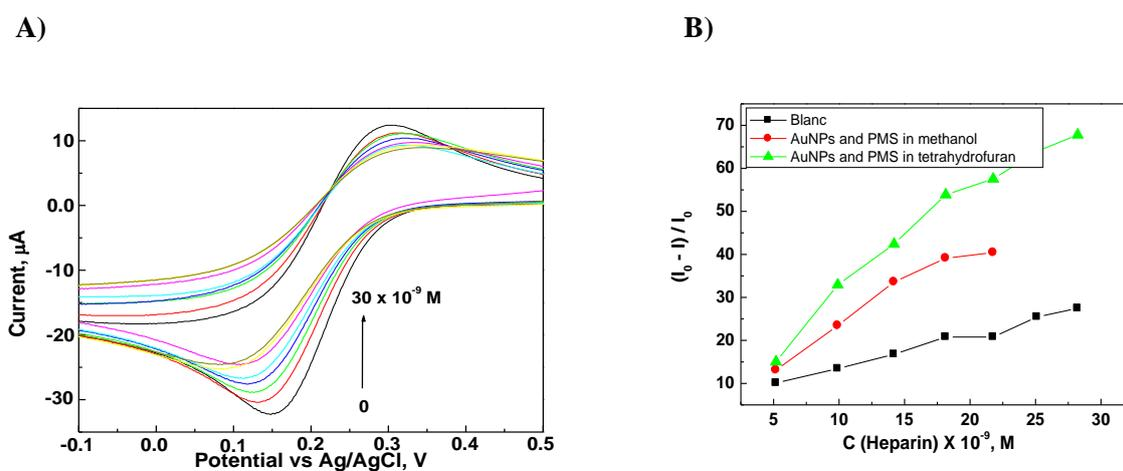
**Figure 7.** A) Cyclic voltammograms obtained with the polymethinium salt/AuNPs/plasticized PVC-modified carbon electrode in  $10^{-3}$  mol  $L^{-1}$   $K_3Fe(CN)_6$  after the addition of different concentrations of
