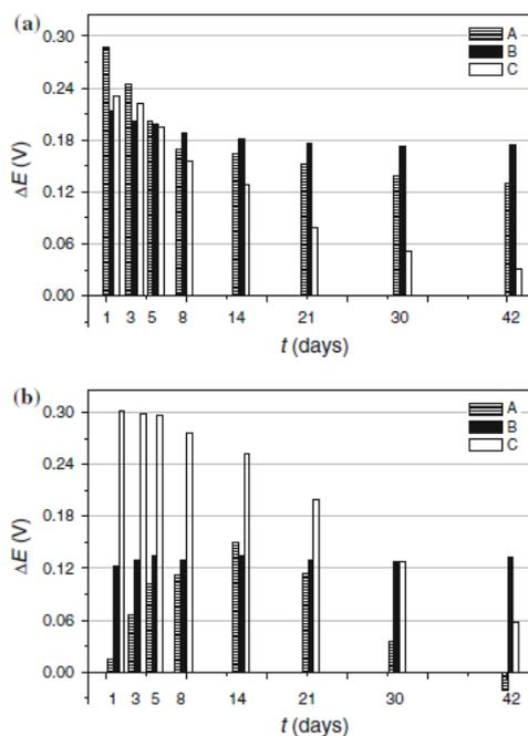
**Fig. 3** Influence of postpolymerization treatment of electrodes based on poly(neutral red) (PNR) (a) and polyaniline (PANI) (b) on their long-term stability in 0.001 M sodium citrate dissolved in 0.02 M TRIS with 0.1 M  $\text{KNO}_3$  at pH 8.5: (A) no treatment, (B) at constant potential vs Ag/AgCl, (C) dried at 60°C for 2 h ( $n = 3$ )
