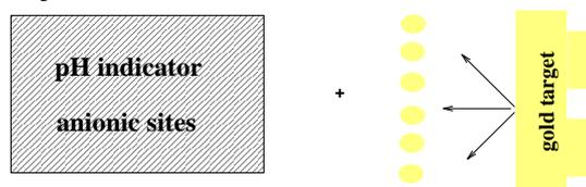
**2nd STEP: evaporation of MPBA and interaction with Au layer deposited onto membrane surface**
