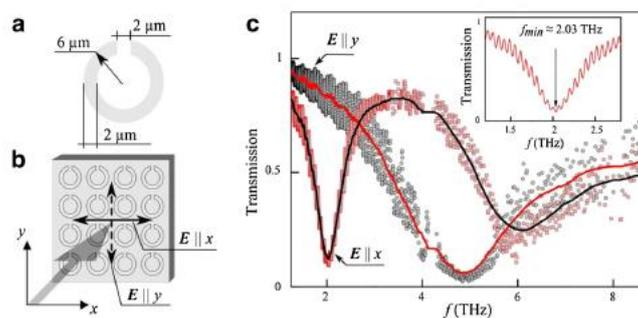
**Fig. 1** **a** Design and dimensions of the split-ring resonators. **b** Experimental geometry: SRRs are oriented in the  $x$ - $y$ -plane. The spacing between the centers of two neighbored rings in both  $x$ - and  $y$ -direction is  $15 \mu\text{m}$ . *Dashed* and *full lined arrows* indicate orientations of the radiation's polarization in parallel to  $x$ - and  $y$ -direction. Transmission was
