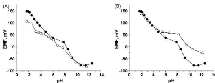
Fig. 1. pH dependence of the potentiometric response for (A) CPP-based membrane in the absence (●) and presence (○) of  $10^{-3}$  M sodium salicylate, (B) CPP-based membrane in the absence (●) and presence (Δ) of anionic sites (13.8 mol% NaTPB relative to receptor).
