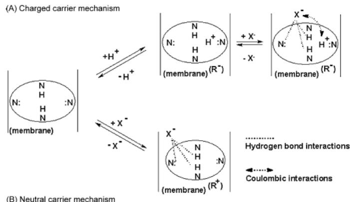
Scheme 2. Possible mechanism of the potentiometric response seen for CPP-based membranes, showing how this receptor system can act as either a singly charged (A) or neutral (B) carrier at pH 5.5 ( $X^-$ , analyte anion;  $R^-$  and  $R^+$  are added lipophilic anionic and cationic sites, respectively).
