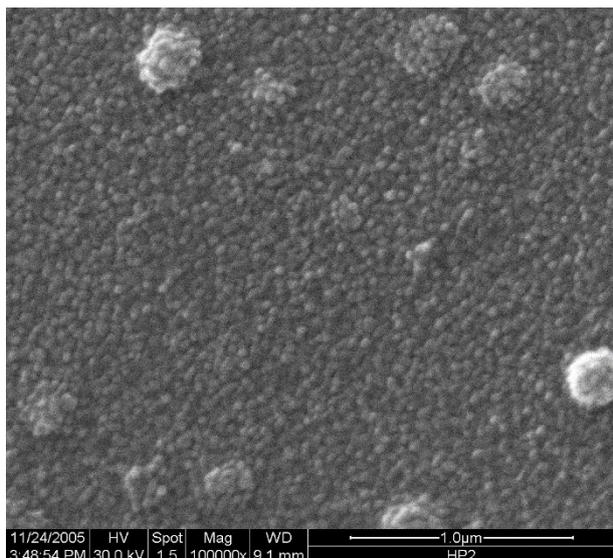
**Figure 2.** Morphology of PANI film deposited onto NPOE-plasticized PVC membrane with PVC : NPOE ratio of 2:1.
