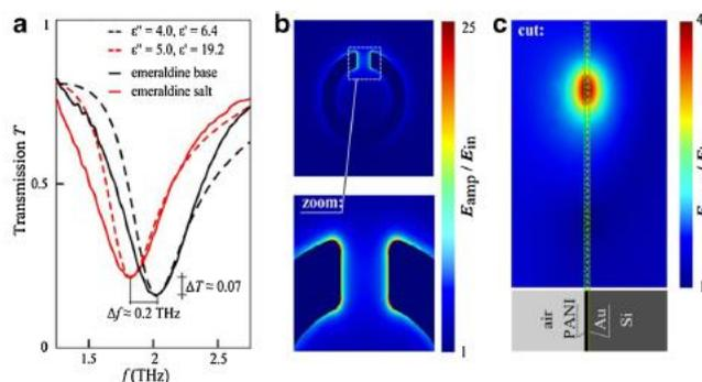
**Fig. 2** **a** Black curves—transmission spectra of an array of split-ring resonators coated by polyaniline in the form of *low conducting* emeraldine base. Red curves—transmission spectra measured in the presence of HCl. The spectrum is red-shifted due to the interaction with gaseous hydrogen chloride resulting in conversion of emeraldine base into the *highly conducting* emeraldine salt. Solid lines shows measured spectra, dashed lines correspond to the results of computer simulation.
