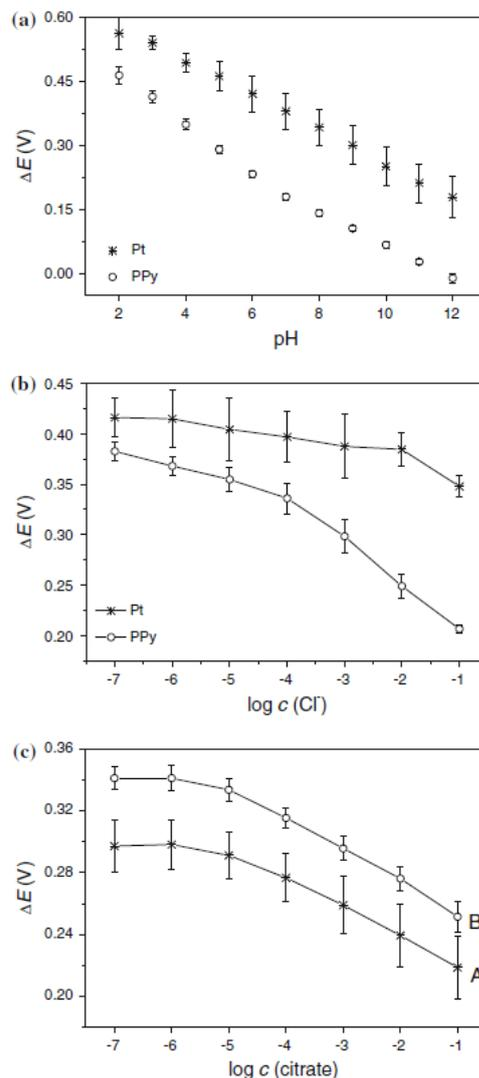
Fig. 2 Dependence of potentiometric responses of bare (Pt) and polypyrrole (PPy)-coated platinum electrodes on pH (a) and chloride concentration (b). Dependence of potentiometric responses of poly(neutral red) electrode with inhomogeneous (curve A) and homogeneous polymer film (curve B) on citrate concentration (c); standard deviation expressed as error bars,  $n = 4$
