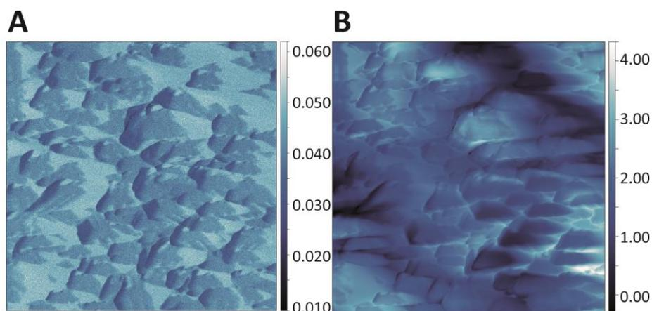
**Figure 5.** SNIM images  $5 \times 5 \mu\text{m}$  of the Au electrode surface. Mechanical amplitude signal (A) and optical signal (B).
