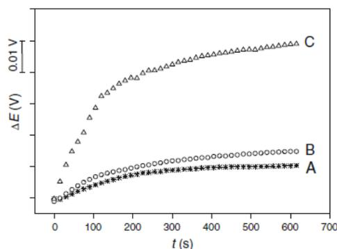
**Fig. 1** Stability of the potential of bare platinum electrode measured in 0.05 M MES solution at pH 5.5 after polishing with alumina (A), burning out in oxidative (B) and reductive (C) part of the flame. For more facile comparison, the curves are adjusted to the same initial point
