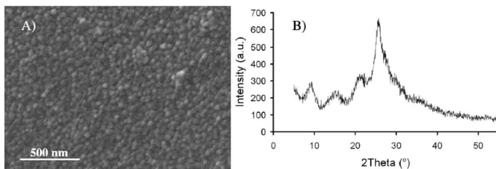
Fig. 1. A) SEM image and B) X-ray diffraction pattern of PANI layer deposited on the surface of the PVC membrane.
