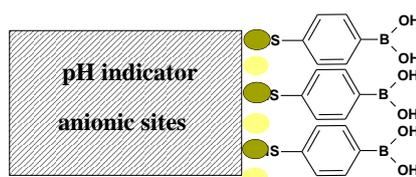
**Scheme 12.** Representation of the modification process of pH-sensitive transducer for potentiometric detection of neutral saccharides.
