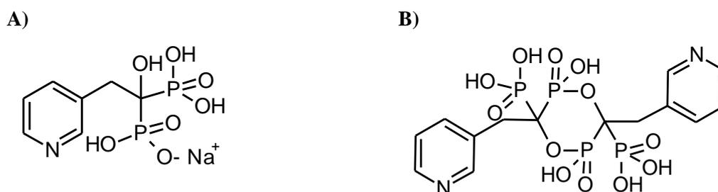
**Scheme 6.** Chemical structures of sodium risedronate (A) and its specific contaminant (B).
