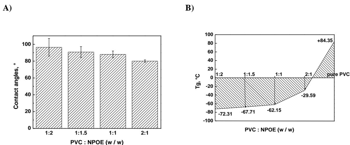
**Figure 1.** Effect of plasticizer content on (A) water contact angle and (B) glass transition temperature ( $T_g$ ) of NPOE-plasticized PVC membrane.
