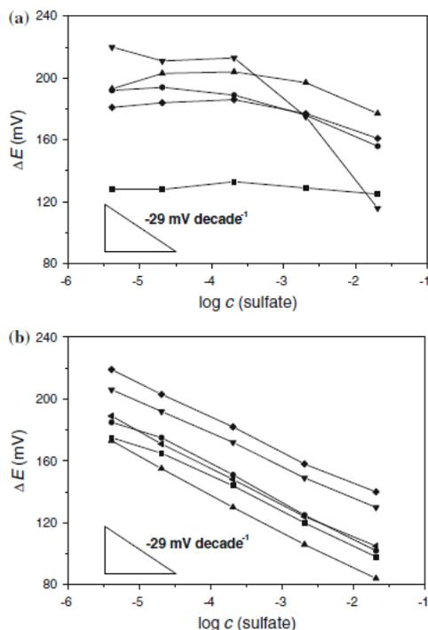
**Fig. 5** Potentiometric responses of TDDMACl-based membrane (PVC/NPOE mass ratio 2:1 and 3 wt. % of TDDMACl) uncoated (a) and coated (b) with the PANI film toward sodium sulfate in time: filled square fresh membrane; after filled circle 1 day, filled triangle 7 days, filled left pointing triangle 10 day, filled inverted triangle 18 days, filled diamond 35 days. Membranes were conditioned in 0.1 M  $\text{Na}_2\text{SO}_4$  before these measurements were carried out
