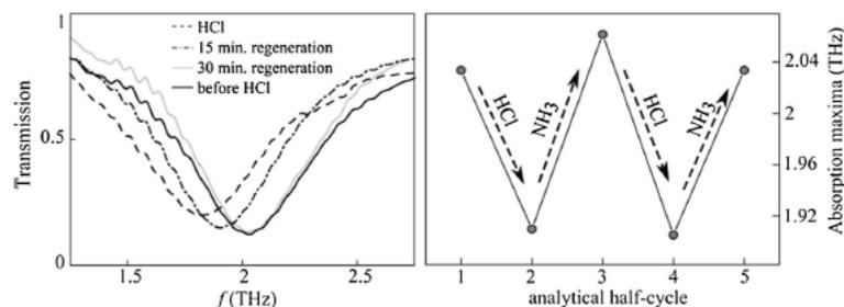
Fig. 3 Sensor regeneration by temperature and by chemical treatment. Left panel shows time-dependent recovery of the samples due to heating: The resonance shifts almost back to its starting position shown by the dashed line. Right panel depicts recovery of the transmission spectrum of
