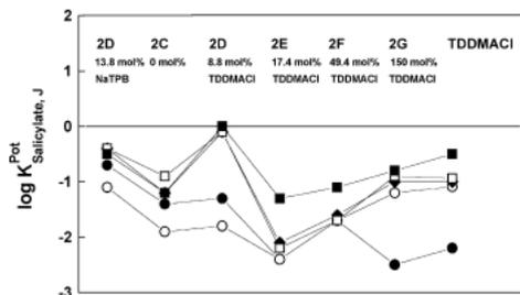
Fig. 2. Plot showing the potentiometric anion selectivity,  $\log K_{\text{Salicylate},J}^{\text{Pot}}$ , of the CPP-based membranes containing various concentrations of anionic and cationic sites at pH 5.5. ( $\text{F}^-$  (●),  $\text{Cl}^-$  (○), benzoate (■), lactate (□), acetate (◆)). <sup>a</sup>All values of the potentiometric selectivity coefficients were obtained using MPM, as detailed in Section 2.3.
