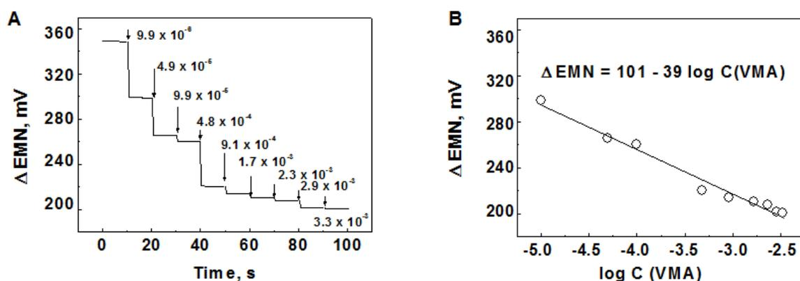
**Figure 6.** (A) Potentiometric response and (B) calibration graph of an electrode modified with a polymer based on a Tröger's base towards VMA in  $0.1 \text{ mol L}^{-1}$  phosphate buffer at pH 7.
