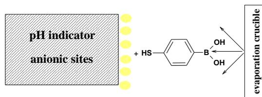
**3rd STEP: covalent bonding of MPBA via thiol group with Au layer adsorbed onto membrane surface**
