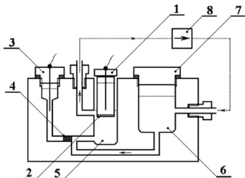
Fig. 2. Schematic representation of the potentiometric cell. (1) Internal reference electrode (Ag/AgCl electrode (0.05 M Tris buffer (pH 7)+0.01 M MgCl<sub>2</sub>+0.001 M EDTA)); (2) probe-immobilized PVC membrane; (3) external reference electrode (Ag/AgCl electrode (0.003 M KCl)); (4) diaphragm (porous ceramic roller); (5) measuring chamber; (6) dosing chamber; (7) screw cap; (8) peristaltic pump.
