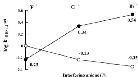
Figure 2. Response selectivities for PVC-membranes based on receptors 1 (open circles) and 2 (closed circles) for OH<sup>-</sup> relative to halides (i.e., log  $k_{\text{OH}^-/J^{\text{sel}}}$ , where  $J = \text{F}^-$ ,  $\text{Cl}^-$ , and  $\text{Br}^-$ ) at pH 9.0. In these experiments, the selectivity factors (log  $k_{i/j^{\text{sel}}}$ ) were determined using the matched potential method<sup>17</sup> as described in the text.
