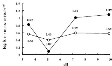
Figure 3. Response selectivities and pH effects for PVC-membranes based on receptors 1 (open circles) and 2 (closed circles) for H<sub>2</sub>PO<sub>4</sub><sup>-</sup> vs HPO<sub>4</sub><sup>2-</sup> relative to F<sup>-</sup> (i.e., log  $k_{\text{F}^-/\text{H}_2\text{PO}_4^-}(\text{HPO}_4^{2-})^{\text{sel}}$ ). In these experiments, the selectivity factors (log  $k_{i/j^{\text{sel}}}$ ) were determined using the matched potential method<sup>17</sup> as described in the text.
