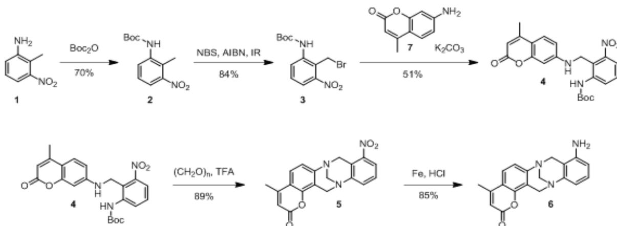
**Scheme 9.** Stepwise preparation protocol of Tröger base functionalized with amino- and coumarin-units **6**.
