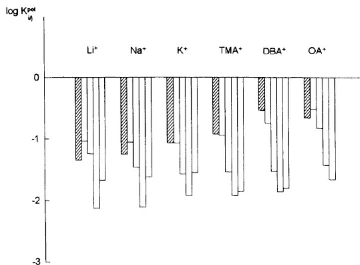
Figure 2. The influence of the host structure on potentiometric selectivity of ISEs reversible to dodecyltrimethylammonium (the bars on chart correspond to hosts: no-carrier, NaTPB, DB18C6, MO5, MO7, left to right; TMA<sup>+</sup>-trimethylammonium, DBA<sup>+</sup>-dibutylammonium, OA<sup>+</sup>-octylammonium).
