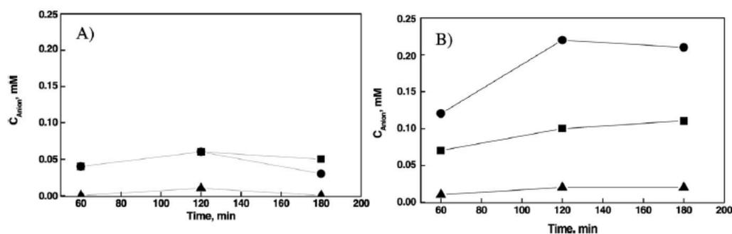
Fig. 2. Time dependence of concentration in the acceptor solution for  $\text{SO}_4^{2-}$  (full circles),  $\text{Cl}^-$  (full squares),  $\text{NO}_3^-$  (full triangle) diffused through uncoated (A) and the PANI-coated (B) membranes.
