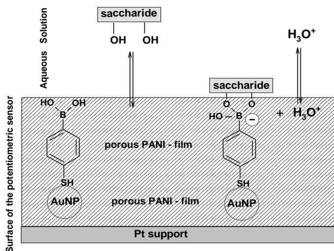
**Scheme 10.** Complexation of diols with phenylboronic acid and formation of potentiometric response.
