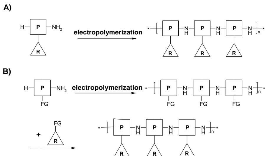
**Scheme 8.** A) Polymerization of receptor **R** with polymerizable unit **P**. B) Introduction of receptor **R** using chemical post-modification of electrochemically generated polymer bearing protected function group **FG**.
