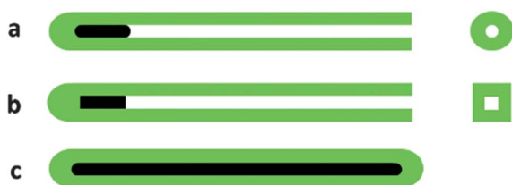
Fig. 8 (a) Soft or (b) hard templates (black) start the growth of PPy (green) nanotubes with circular or rectangular profile, respectively. (c) The core-shell nanotubular structure may be produced by coating of suitable hard templates with conducting polymers.
