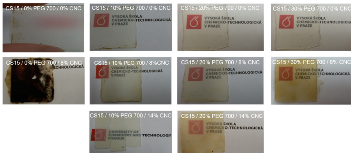
Fig. 5. CS15/PEG/CNC specimen prepared by freeze drying followed by compression molding.
