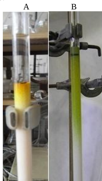
Figure 12 Comparison of color ion-exchange columns after sorption \text{Cr}^{\text{VI}} . A - resin with trimethylammonium functional groups, B - resin with aminomethylglucitol functional groups
