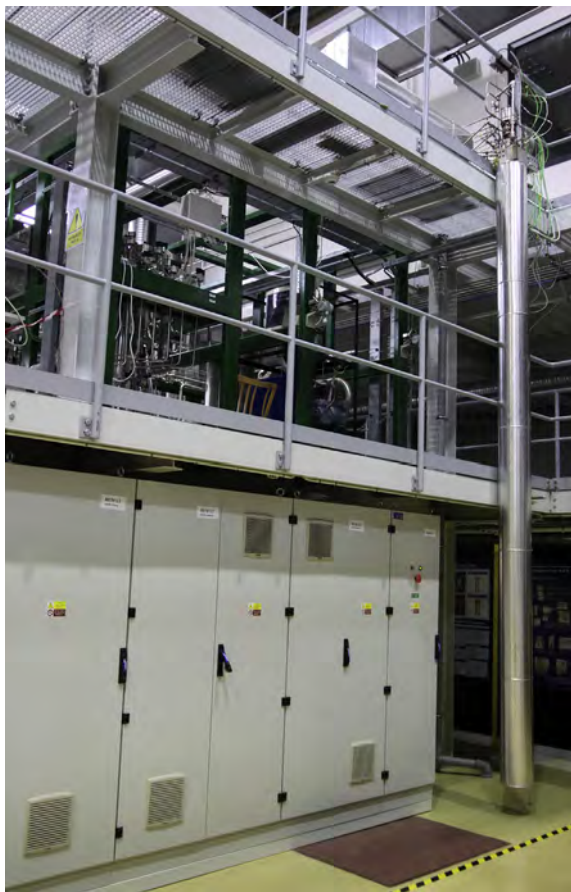
Fig. 5. High temperature helium loop – situation in 2013. The vertical tube on the far right serves as the active channel.
