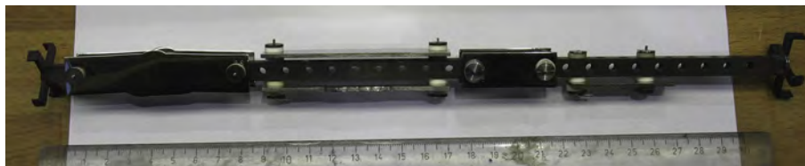
Fig. 9. Set of the holder and corrosion samples before the exposure in HTHL.
