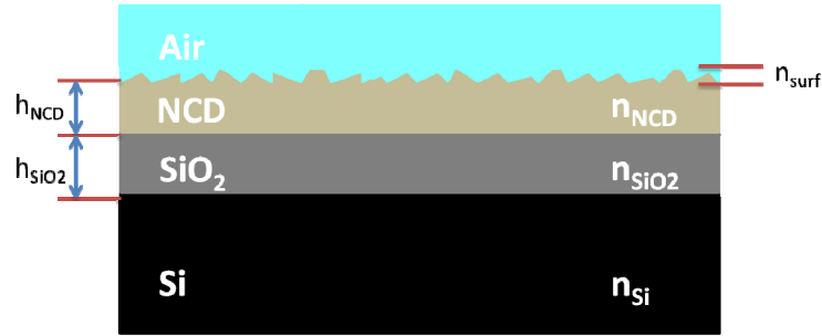
Fig. 2. Schematic view of the optical planar NCD waveguide structure.
